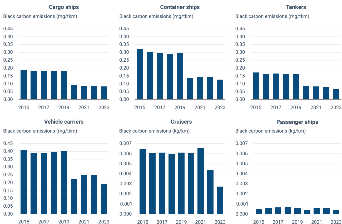
Figure 2.18 BC specific emissions from selected freight and passenger ship types in the EU-27
